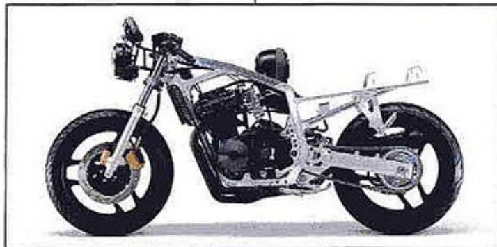
The GSX-R750 frame is extruded aluminum, for remarkable strength and lighter weight.
