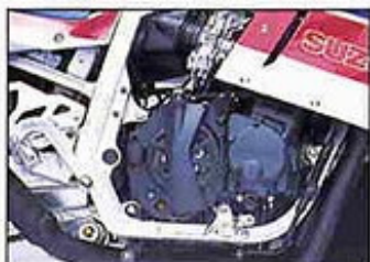
A dry clutch with adjuster gives quick, race-proved response.
